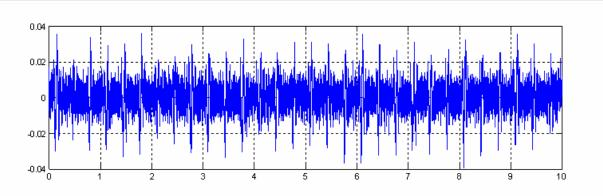
The reconstructed signal by IMFs 1-3 (control sample)
